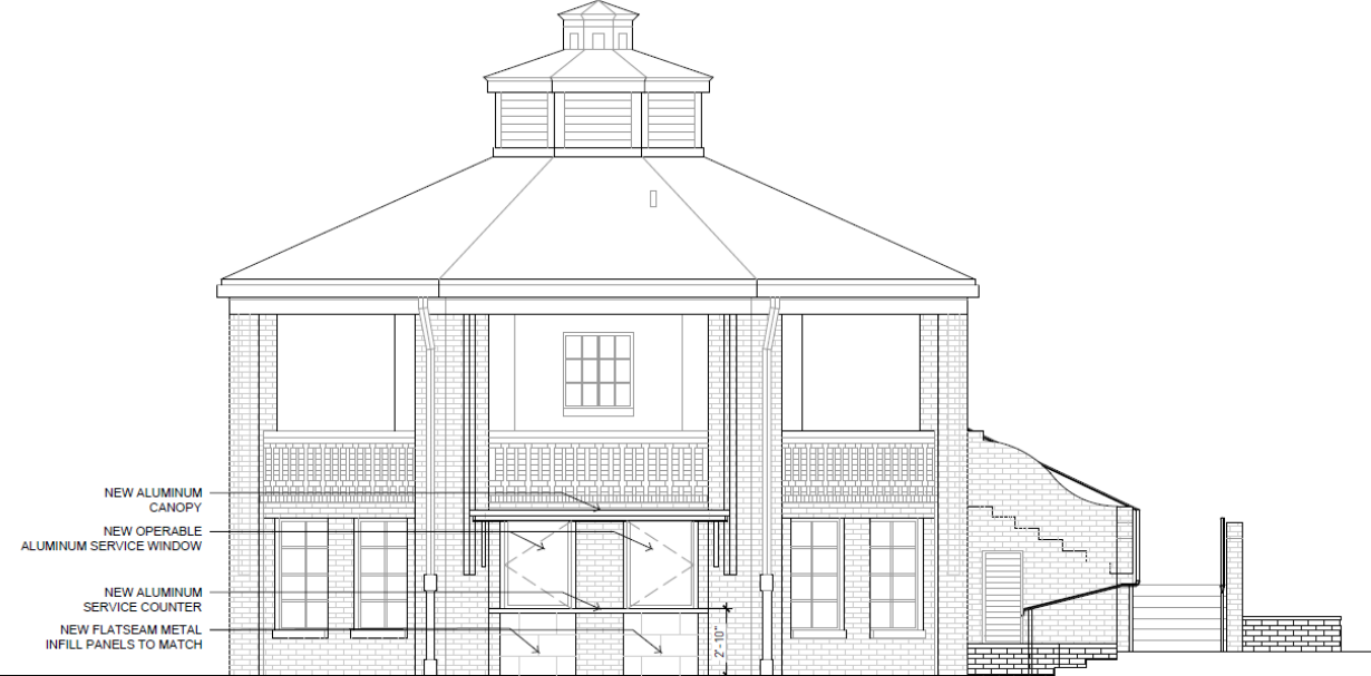
EAST ELEVATION - ALTERNATE SERVICE WINDOW
