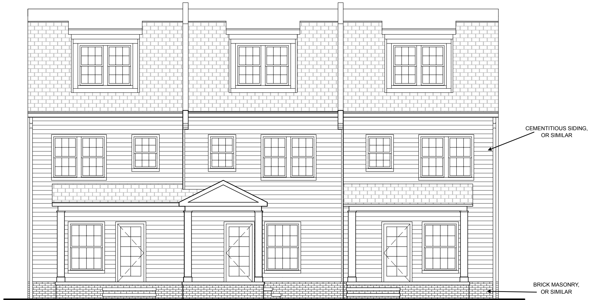
1 SOUTH ELEVATION AT PATTERSON AVE SCALE: 1/4"=1'-0"
