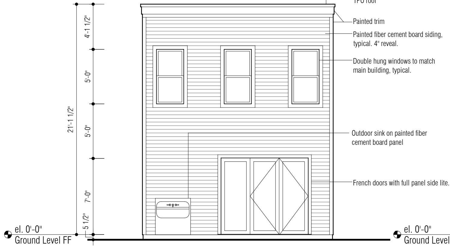
1 Exterior Elevation - West 3/16" = 1' - 0"
