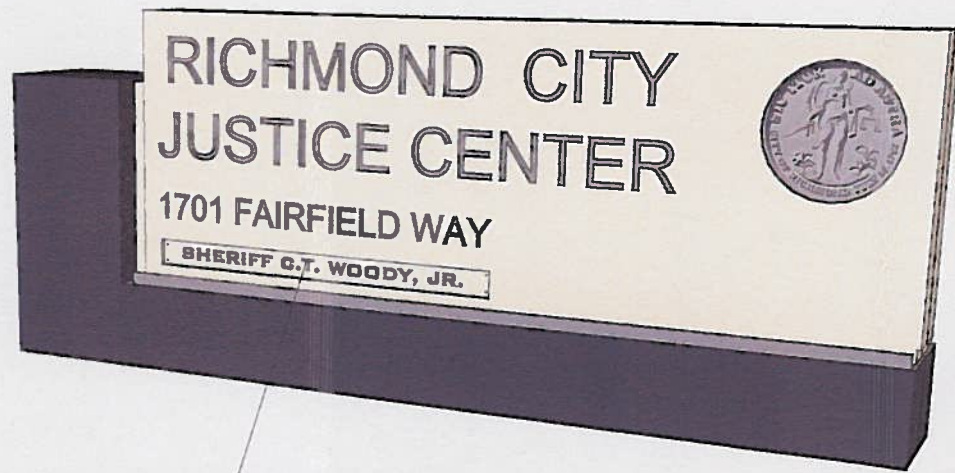
RECESSED CONCRETE PANEL WITH PIN MOUNTED ALUMINUM LETTERING PANEL ATTACHED TO SIGN WITH SECURITY SCREWS
