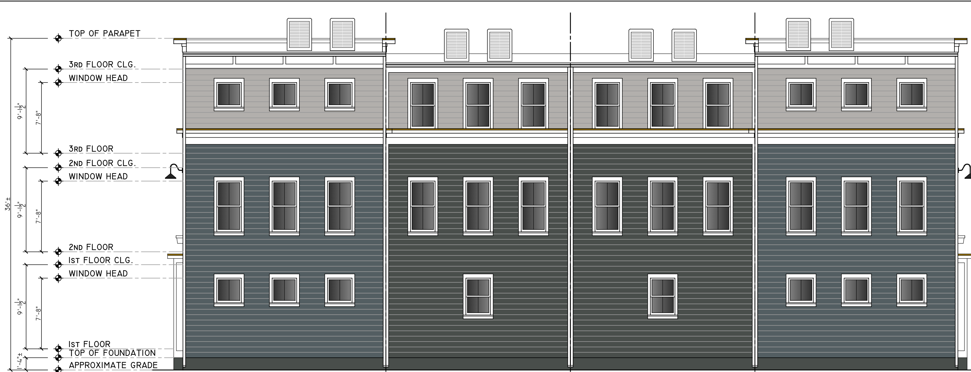
02 | BUILDING B - WEST ELEVATION 3/16" = 1'
