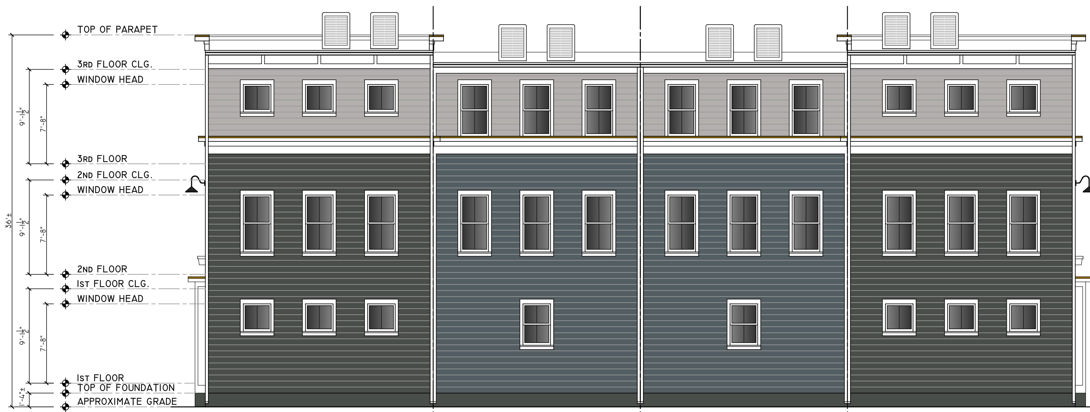
01 | BUILDING A - EAST ELEVATION 3/16" = 1'
