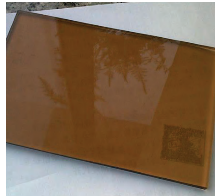
Reflective bronze glass at Infill Addition
