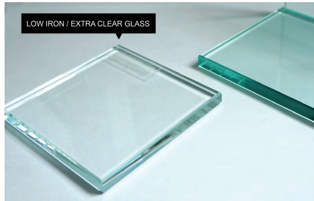
Low iron, ultra clear glass at bridge connection
