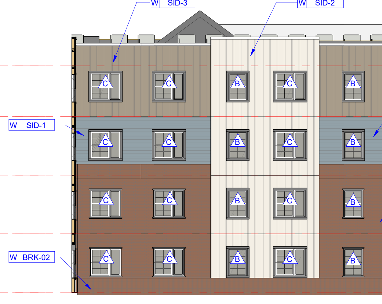
4D ELEVATION - INNER COURTYARD WEST
