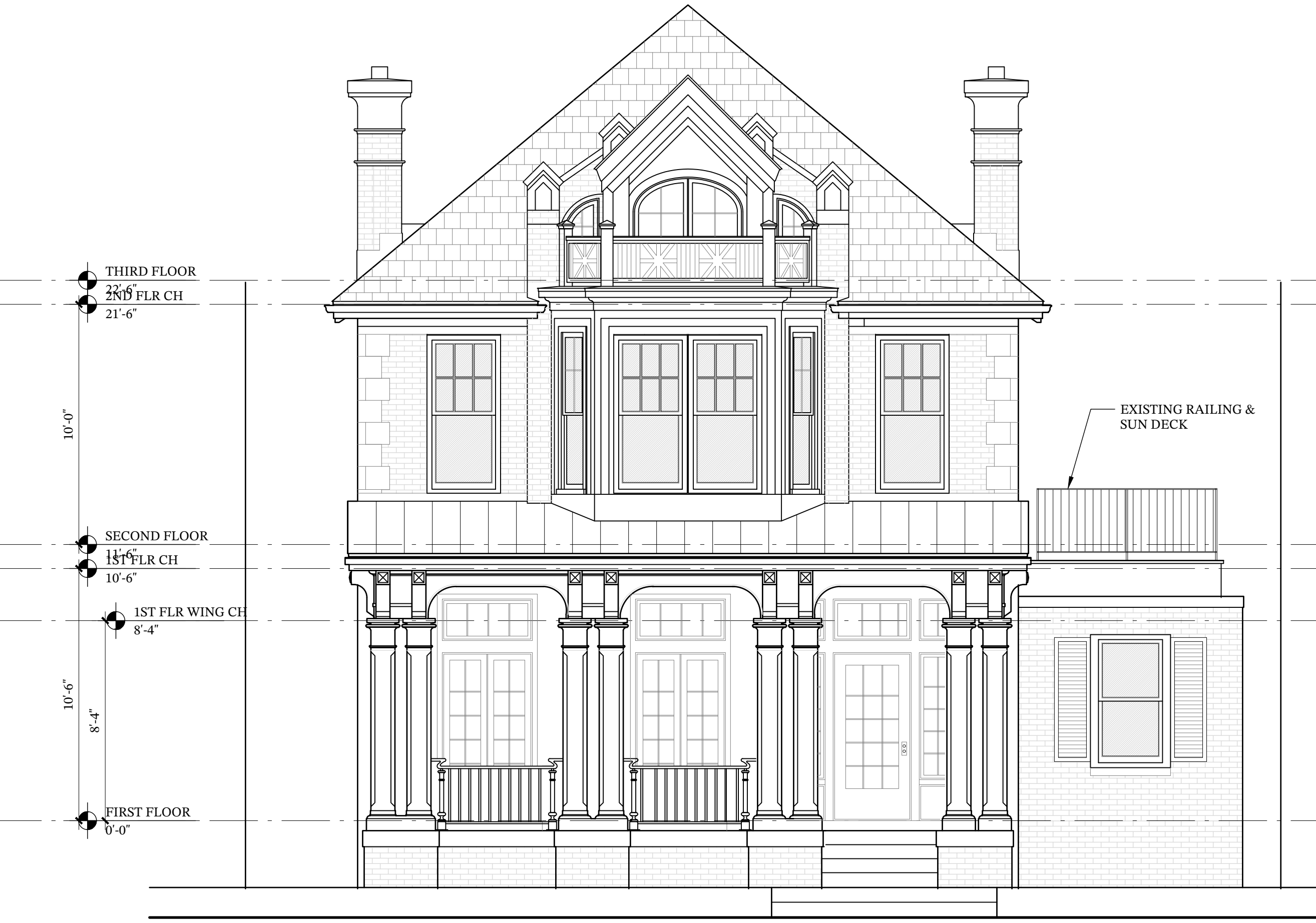
EXISTING NORTH ELEVATION A 1/4" = 1'-0"
