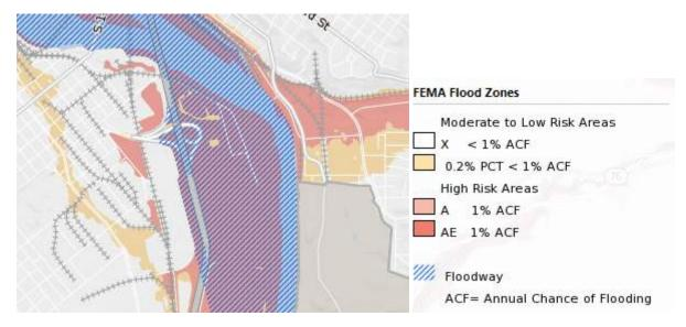
FEMA recently raised the flood levels for the city of Richmond in general which puts the new building in a high risk of flooding. To minimize damage to the installations and interruption of operations, the building is raised one story above grade and the parking spaces are located underneath on the first floor.
