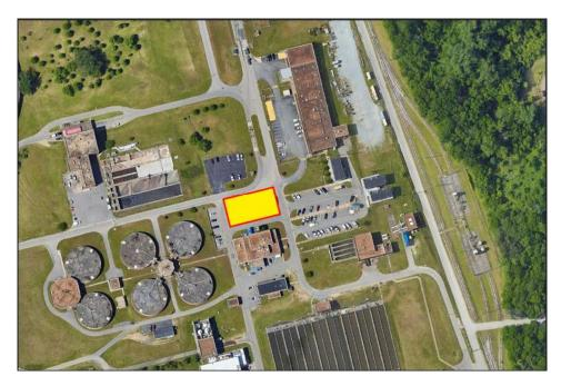
The site of the new Administration building is surrounded by process facilities consisting of both tanks or buildings. Almost all the building present in the plant are square brick boxes that vary in size depending on the process or equipment they house. The tanks are either circular or rectangular, above grade or buried.
