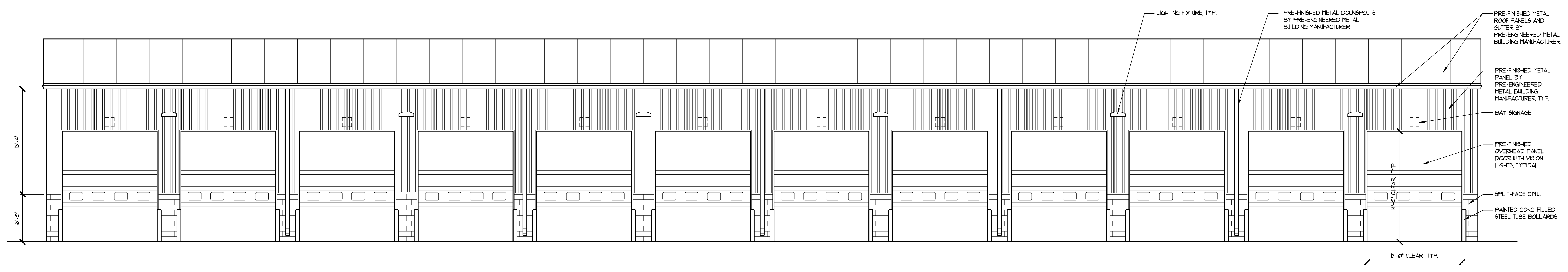
1 BUILDING 2 - NORTH AND SOUTH ELEVATIONS SCALE: 3/16" = 1'-0"
