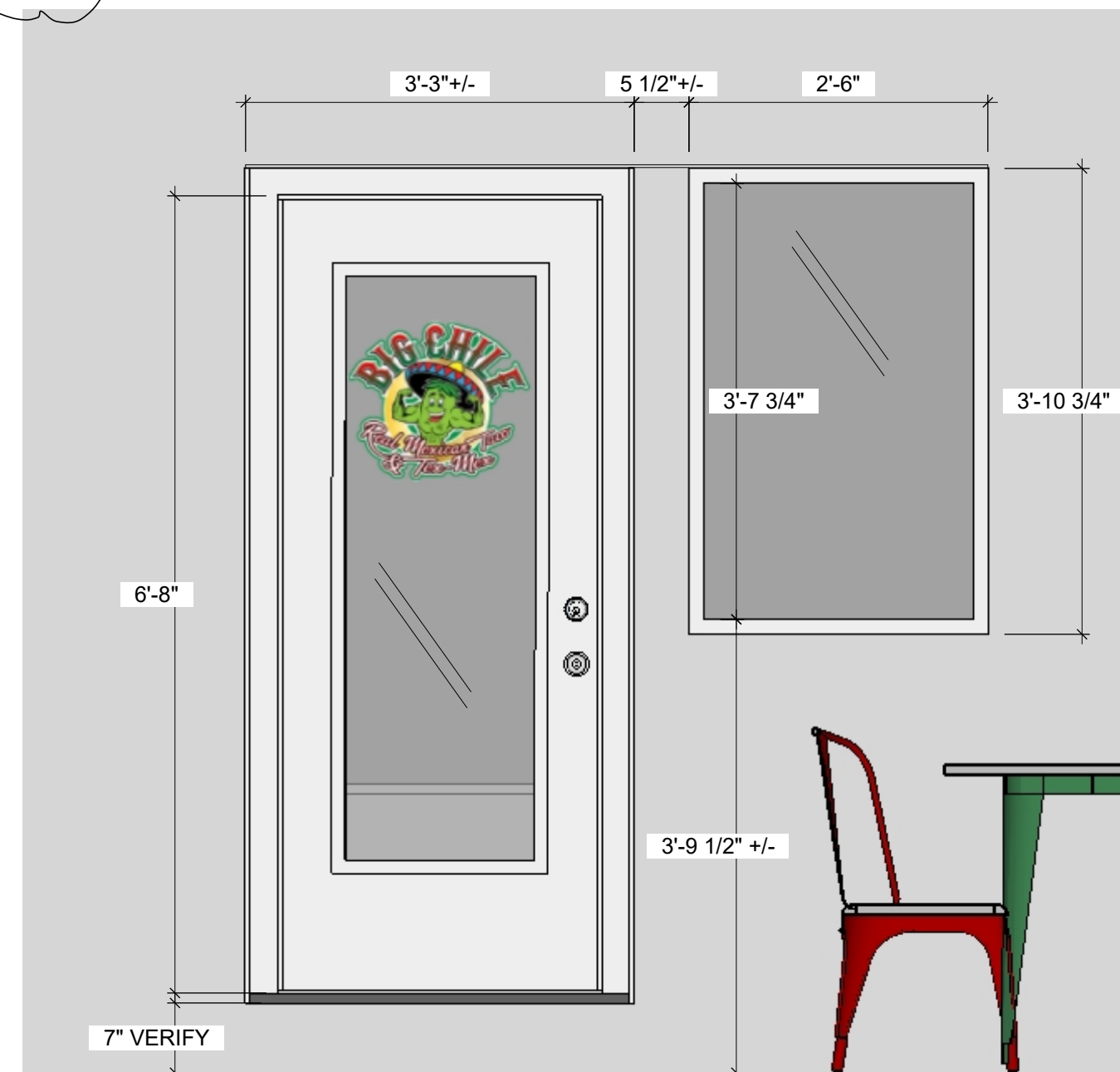
7 A102 NEW DOOR AND WINDOW EXTERIOR ELEVATION SCALE: 3/4" = 1'-0" NOTE: DOOR STYLE TO BE DETERMINED. 1 12/27/24 ELEVATION OMITTED 2 3/3/25 ELEVATION INCLUDED
