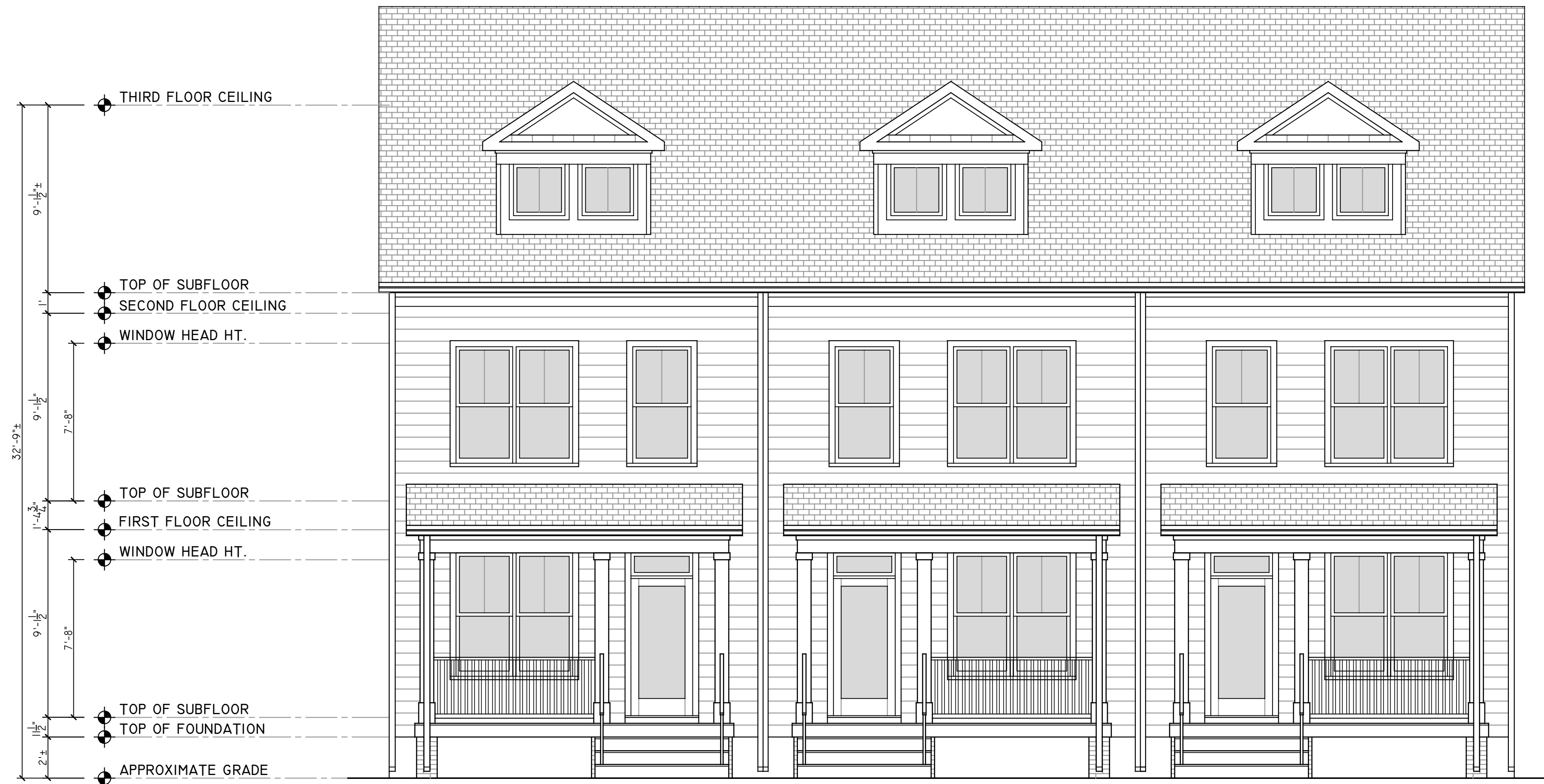
01 | FRONT ELEVATION - BUILDING A 1/4" = 1'
