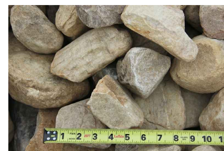
Velocity reducer & trash/salt trap stone type
