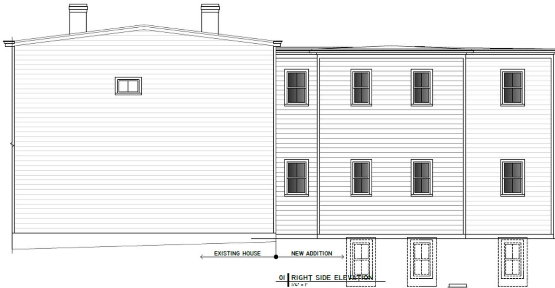
*Proposed Right Elevation Showing New Window Configuration*
