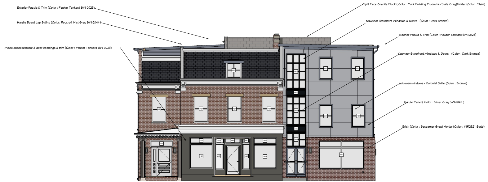
North Exterior Elevation 1/6 in = 1 ft
