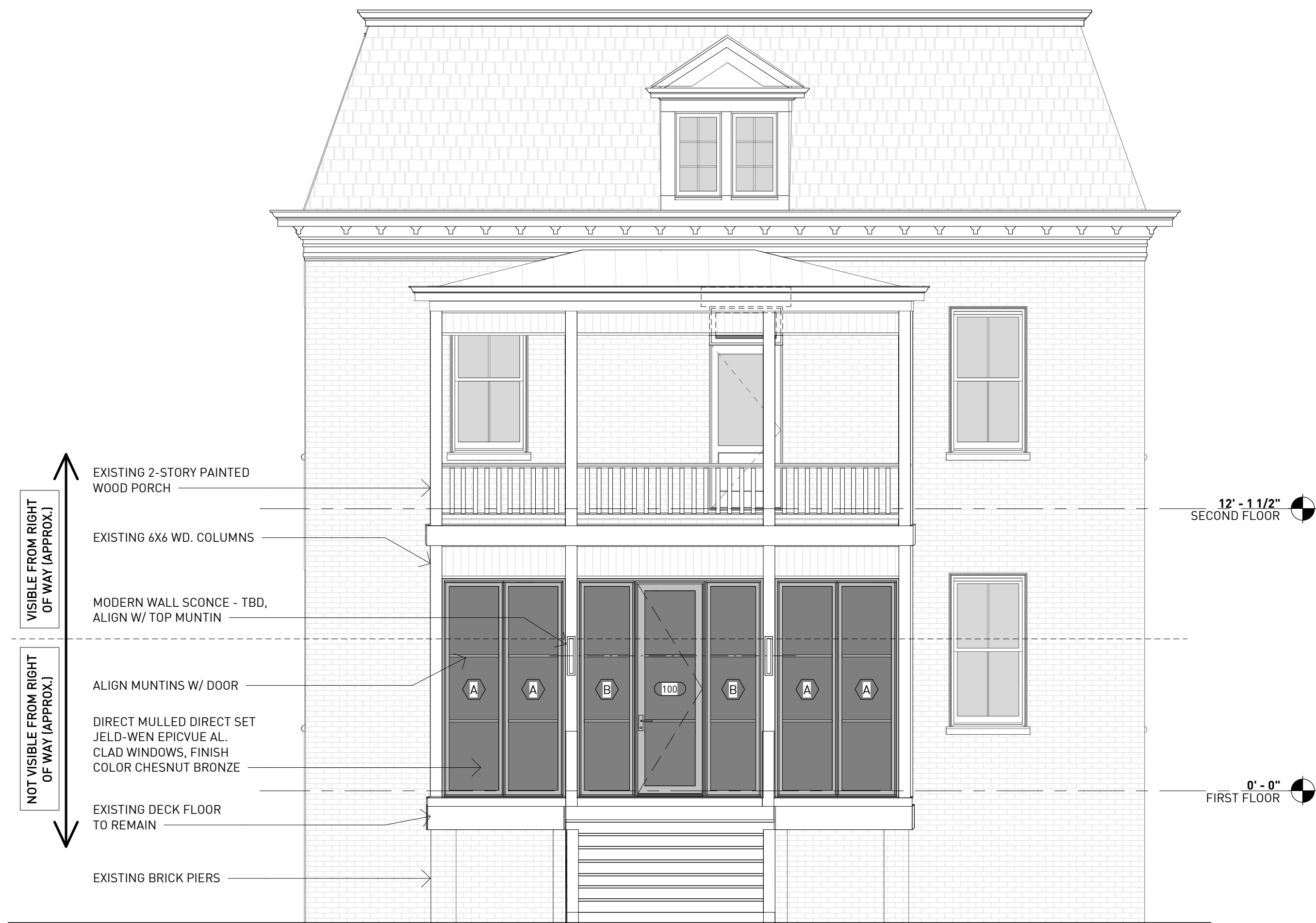
2 PORCH INFILL - NORTH ELEVATION 1/4" = 1'-0"
