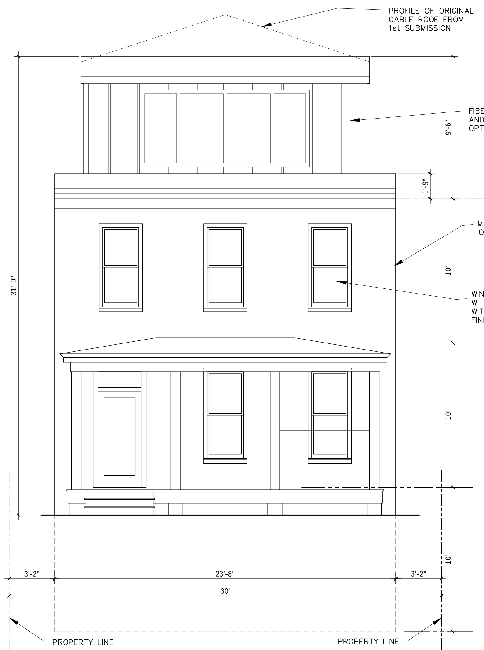
① Front (west) Elevation SCALE: 1/4" = 1'-0"
