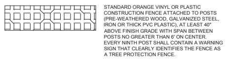
4 TREE PROTECTION AND PRESERVATION NOT TO SCALE VIRGINIA EROSION AND SEDIMENT CONTROL HANDBOOK
