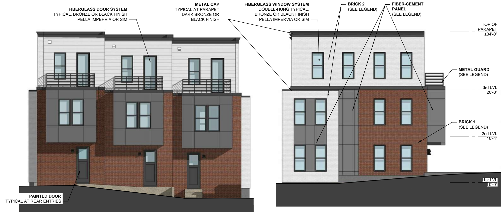
GROUPING #2 | NORTH ELEVATION 2n
