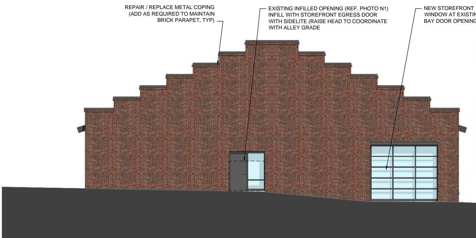
PROPOSED NORTH ELEVATION (FACING PUBLIC ALLEY) 1n
