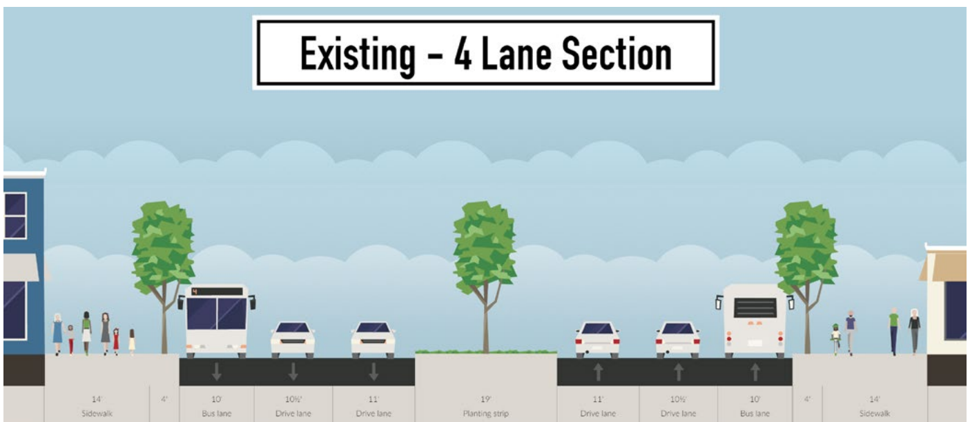
Figure 14: Existing four-lane typical section along Broad Street
