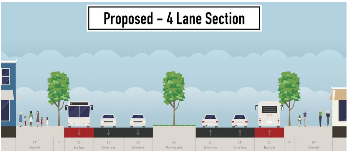
Figure 16: Proposed four-lane typical section along Broad Street
