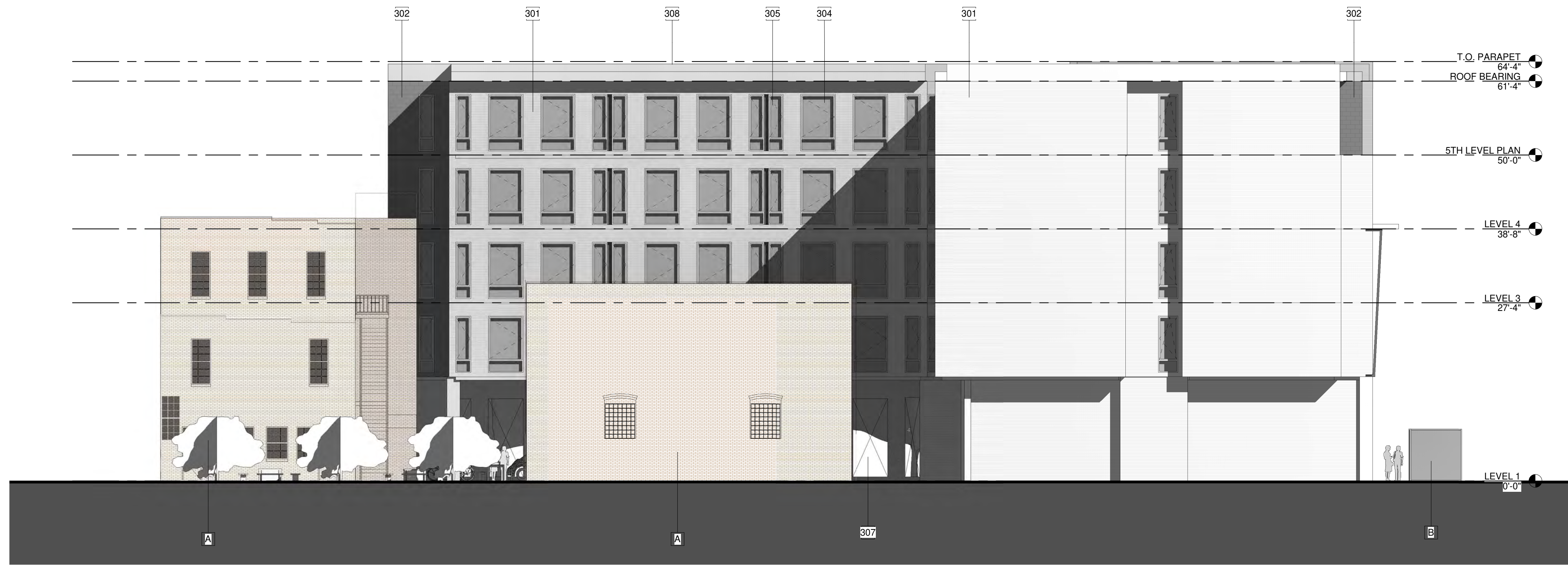
1 NORTH ELEVATION A302 3/32" = 1'-0" 0 16 32 48 FT
