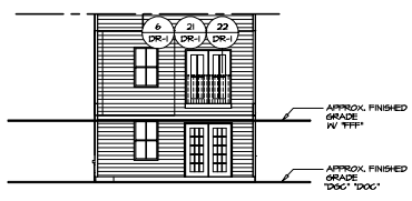
4 PARTIAL REAR ELEVATION SCALE: 1/4" = 1'-0" DOUBLE PATIO DOOR KITCHEN "DPC" DOUBLE PATIO DOOR HALLKIT/BASEMENT "DPC" SHOWN IV EXTERIOR UNIT "SAE"
