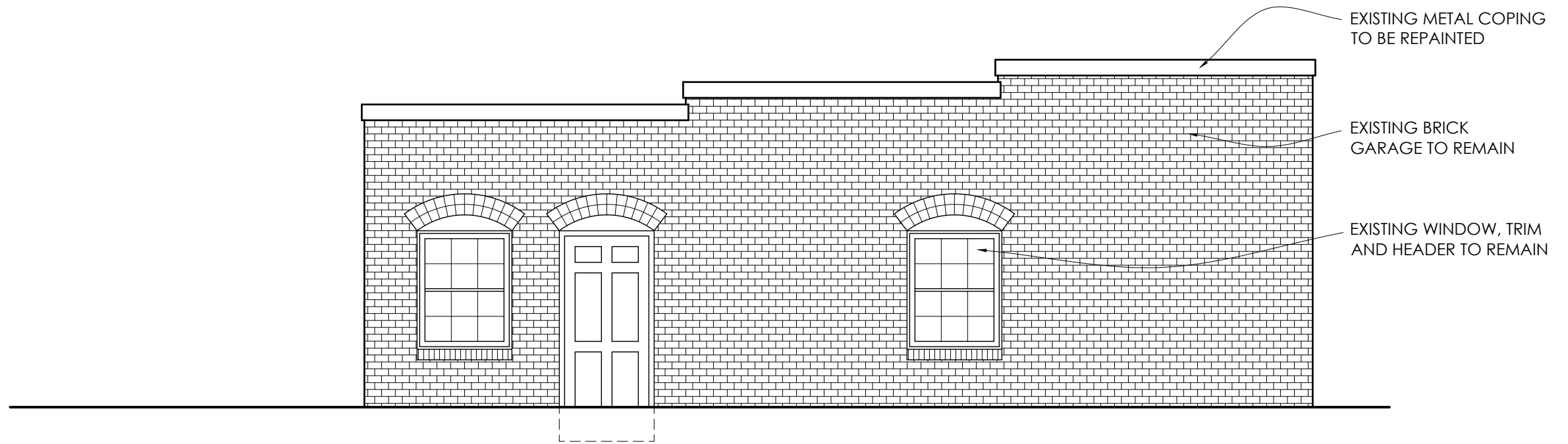
EXISTING SOUTH ELEVATION
