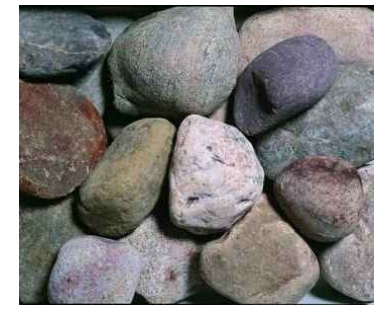
Ornamental gravel for conveyance channels and stabilized outfall: 3-5" Chalet Stone
