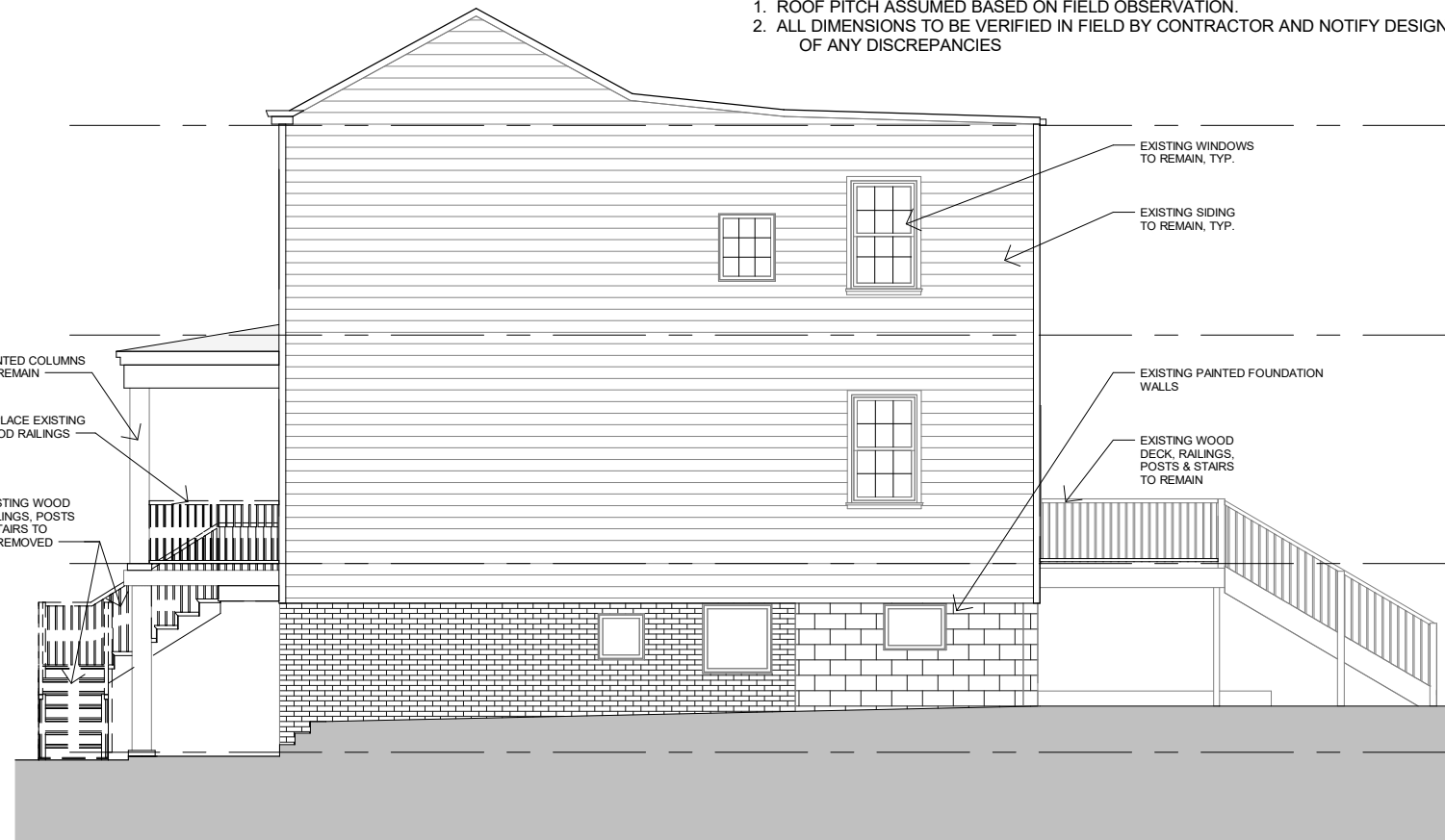
② Existing & Demo East Elevation 1/8" = 1'-0"
