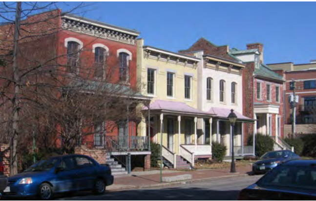
Residential Character -- Porch and entrance at base, vertically and symmetrically arranged openings, and a decorative cornice at top. Subtle variations in height and color, consistent materials.
