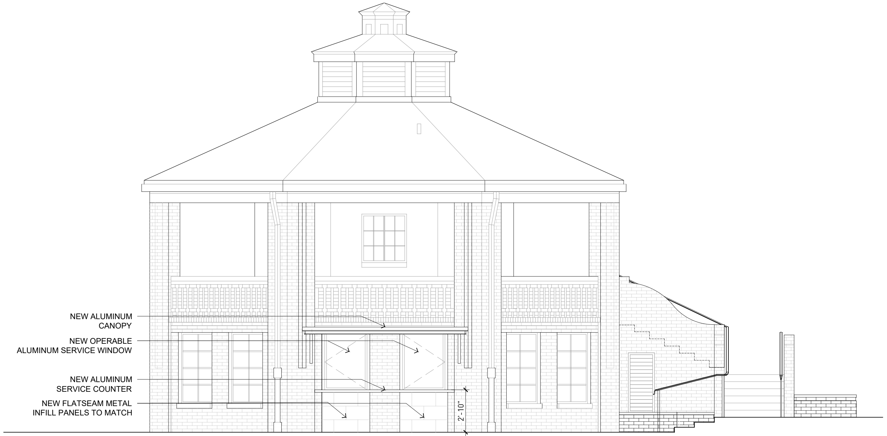
EAST ELEVATION - ALTERNATE SERVICE WINDOW
