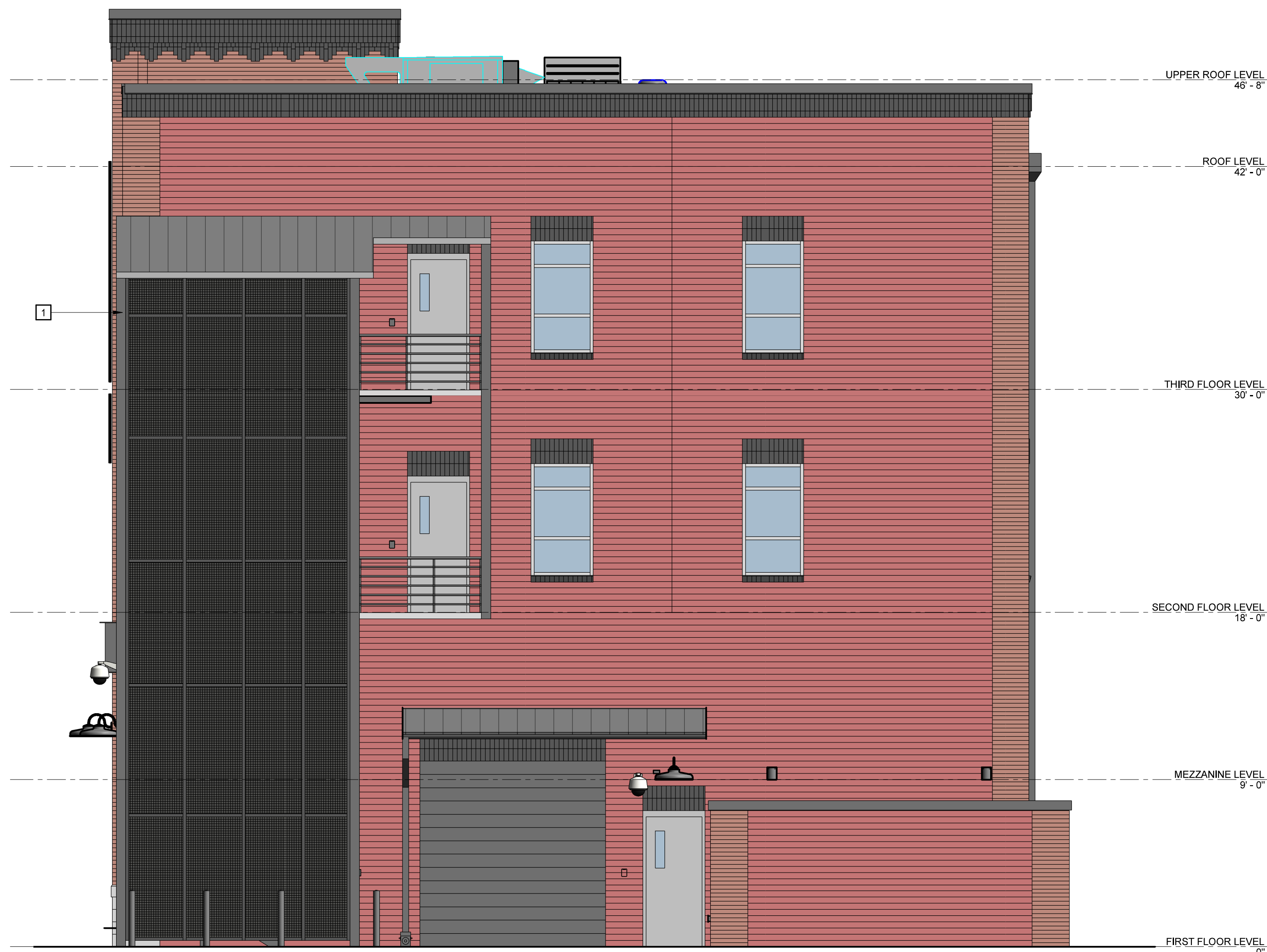
1 SOUTH BLDG ELEVATION A2.1 | A4.1 1/4" = 1'-0" 0' 1' 2' 4' 8' 1/4" = 1'-0"
