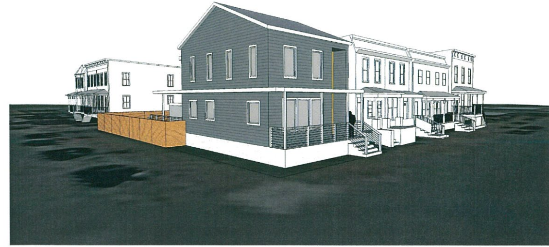
VIEW OF WEST/SOUTHWEST CORNER ON N 29TH STREET AND E LEIGH STREET FRONT FACADE ALIGNS WINDOWS, PORCH AND PORCH ROOF WITH NEIGHBORING HOUSES. WINDOW PATTERNS FROM NEIGHBORS ARE CONTINUED ON E LEIGH STREET FACADE AND N 29TH STREET FACADE. WINDOWS ARE VERTICALLY ALIGNED TO MATCH PROPORTIONS OF NEIGHBORING HOUSES. RESPECTS THE TYPICAL HEIGHT OF SURROUNDING AND NEIGHBORING BUILDINGS.
