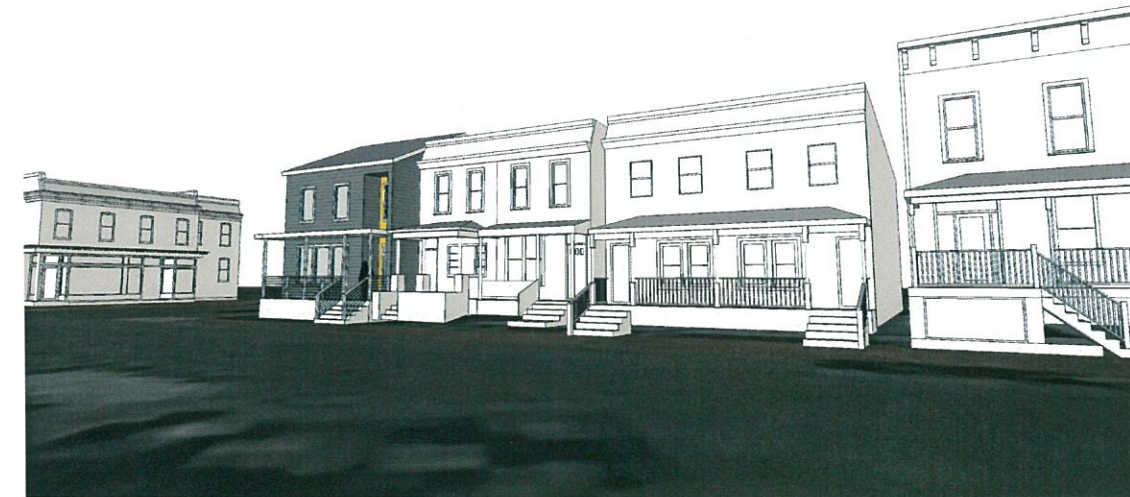
VIEW OF PROMINENT STREET FRONT ALONG E LEIGH STREET HEIGHT OF GABLE ROOF ANCHORS WEST CORNER OF THE BLOCK AND HEIGHT OF 2912 E LEIGH STREET NEWLY CONSTRUCTED HOME ANCHORS EAST CORNER. THE FACADE HEIGHT, FRONT PORCH PROPORTIONS AND WINDOW PLACEMENT ALL RESPECT THE ARCHITECTURAL ELEMENTS ALONG THE STREET FRONT.
