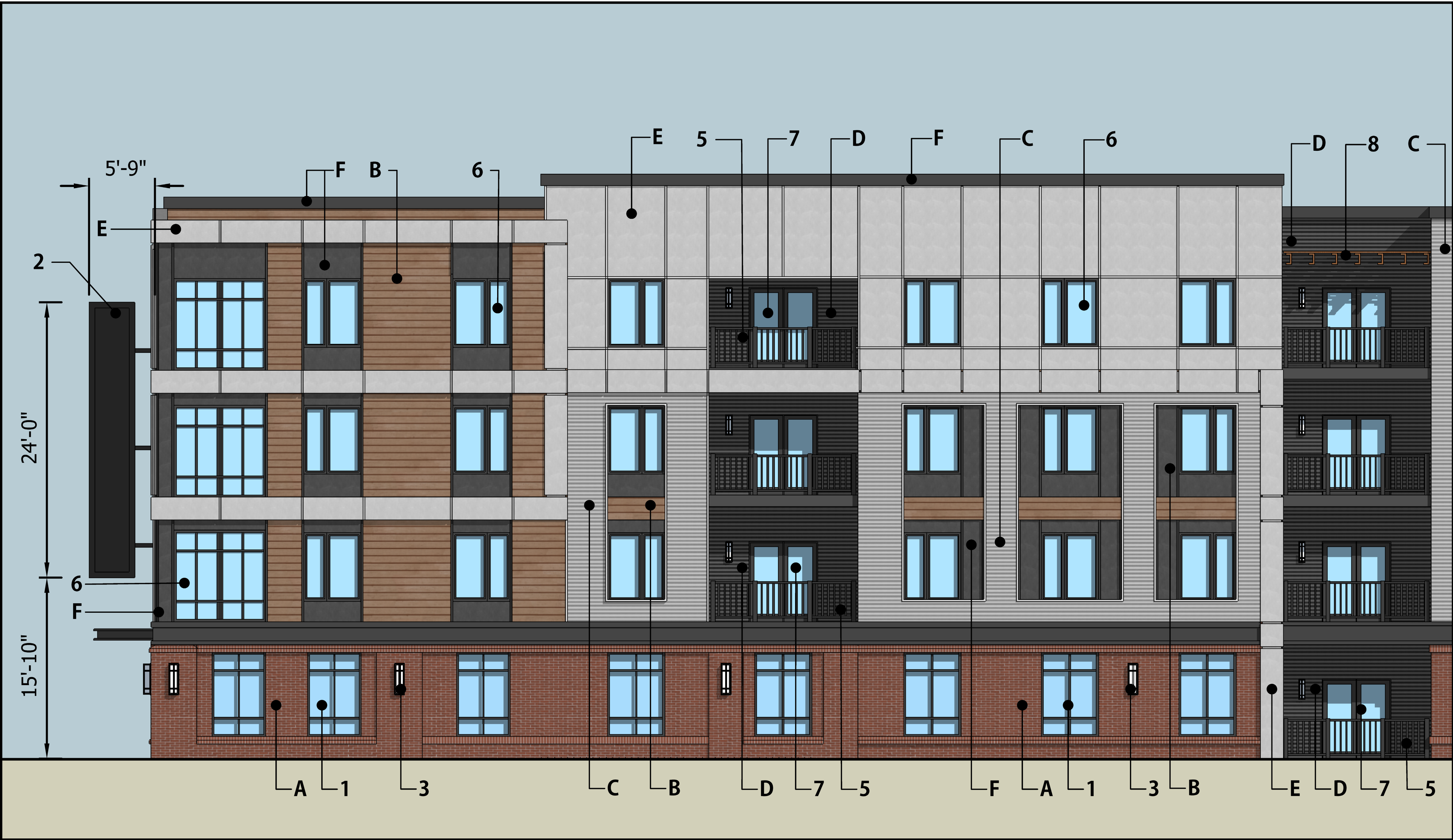
2 ENLARGED EAST ELEVATION PARTIAL / MATERIALS 3/16"=1'-0"
